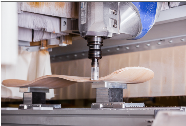
Aluminum vacuum blocks VCBL-A-K2 for clamping solid wood
